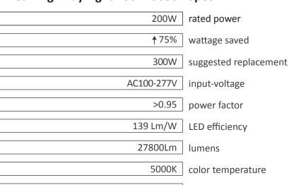
>70 CRI 360 LED quantity damp IP rating 40° / 80° beam angle <15% THD
